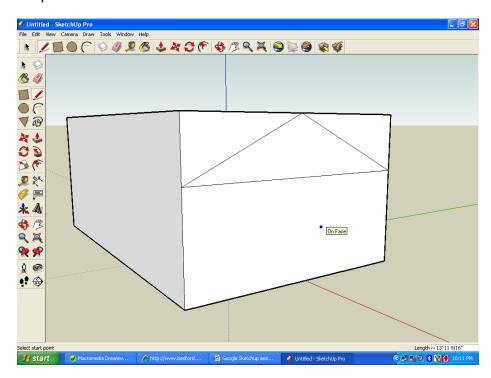
**Step 5:** Use the PUSH/PULL tool to eliminate the extra roof.
