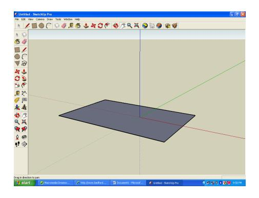
**Step 2:** Use the PUSH/PULL tool to pull the box up to 16 feet tall. Use the TAPE MEASURE TOOL to check your measurements and the PUSH/PULL tool to readjust as needed (the SCALE tool will only make your box crooked).
