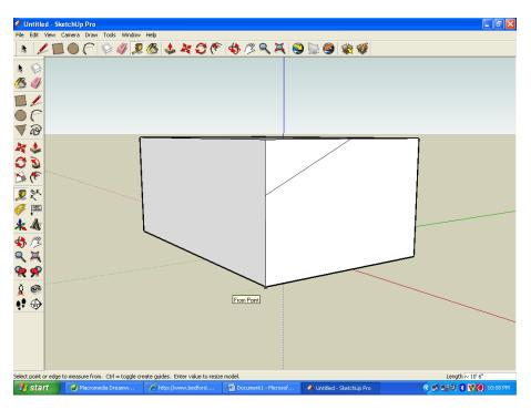
**Step 4:** Draw a line, parallel to the ground, across the house to the other side. Remember, if the line is parallel to the ground it will change to GREEN. Then complete your triangle back up to your midpoint.
