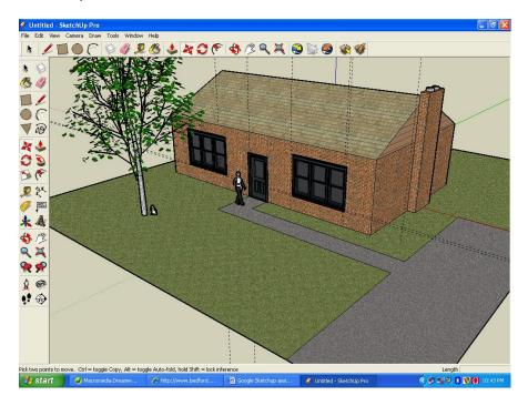
**Step 1:** Create a rectangle. Use the TAPE MEASURE TOOL to see how it measures. Use the SCALE tool to change the size so it measures 40 feet long by 25 feet wide. (You don't have to be too precise- it's okay if you're within one foot).
