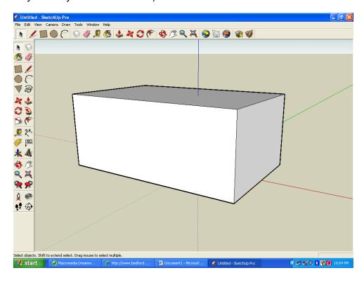
**Step 3:** Use the LINE TOOL to find the midpoint on the side of your roof and draw a diagonal line to one side. The line should be ten feet up the side. Use your TAPE MEASURE TOOL to measure and make sure the lowest point of your roof begins at 10 feet above ground.
